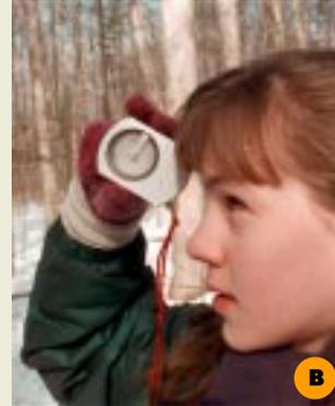
**Trees are measured before they are cut to determine the amount of wood they contain. The tree's trunk diameter (A) and height (B) are measured to estimate the usable wood in a tree.**
